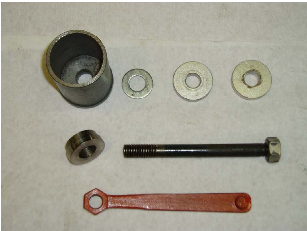
Puller for removing a "stuck" Zenith venturi from the top or bottom casting.
