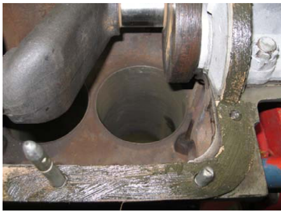
Apply sealant over the rear cap cork
