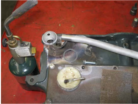
Cleaned parts prior to fluxing
